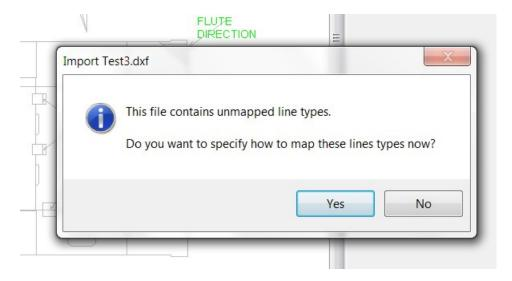
If you elect to map the linetypes, one by one they are highlighted on screen, and you are taken into the standard linetype dialog to pick the appropriate CimPACK linetype to use for the un-mapped linetype from the file. Once all of the linetypes have been cycled through, you get options on what to do.
