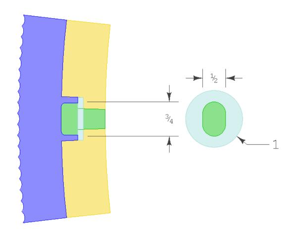
Martin Posilock patterns now shift shell patterns so the horizontal seams are between bolt rows automatically. Also, there is now a configuration for the types of holes to mount the hoops with, whether they should be all circles, all ovals, or a combination. The oval holes will remain as is unless this option is configured.
