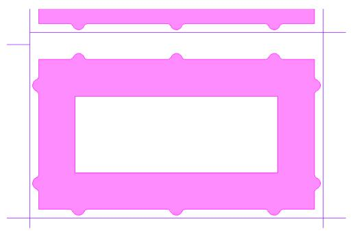
The rubber sheet configuration menu now also sets the default width and offset for each type of rubber, and whether spacer tabs are to be added. Also, 45 additional new rubber types are supported here, linetypes 700-745.
