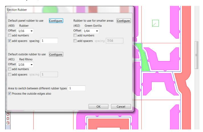
An additional offset was added to ejection rubber for the trail edge, mainly for rotary work. You can then have a large offset on the rear of any shape that is done as a Window, so for pieces that will get "shunted" around the cylinder. Also, an additional shape was added for chopped scrap areas like the below, creating a "U" instead of the full rectangle.
