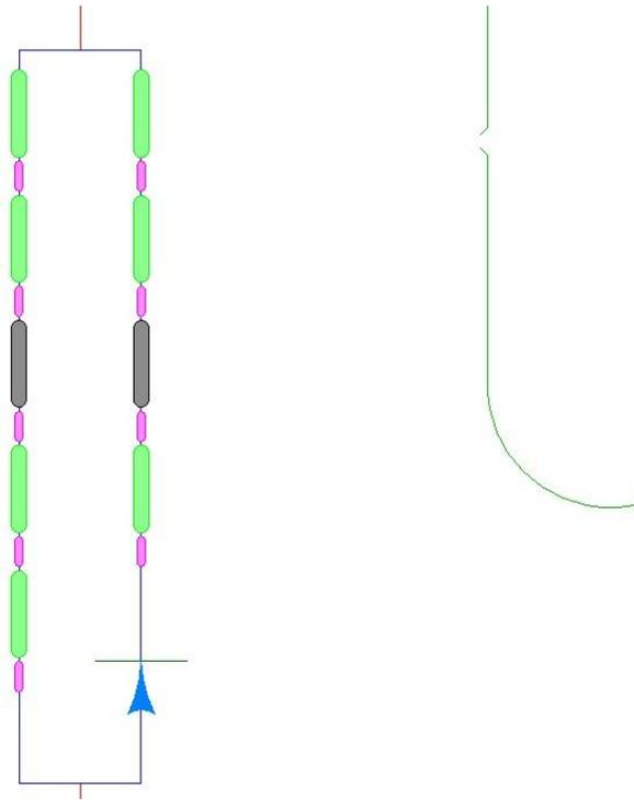
If you leave on the option to split the striprules to the knives, then the teeth close to the striprules are all removed, and the bridging centered between each set of striprules.
