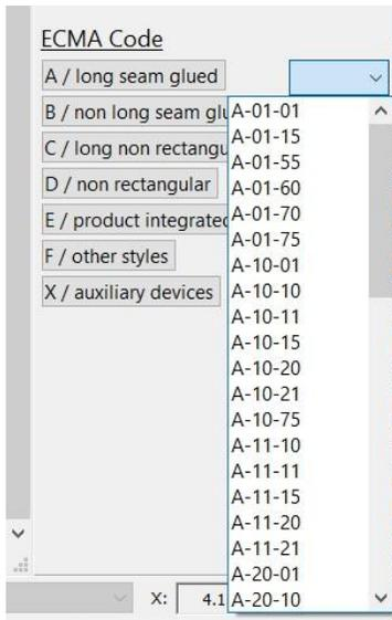
The interface for the Ecma is the same as that of the Fefco library for consistency. Within each category, you can cycle up and down through each pair of designs, with both the flat and 3D images shown.
