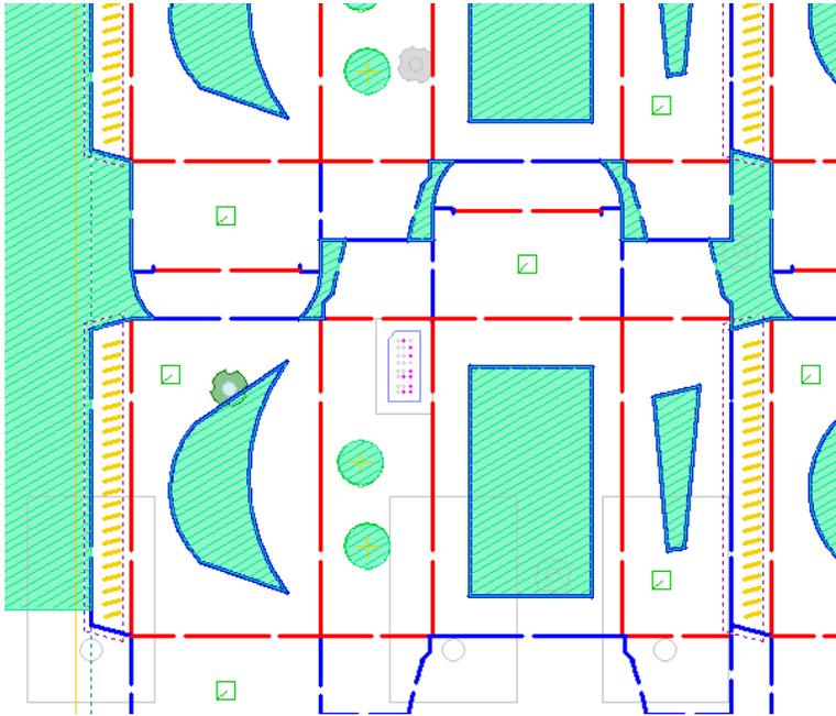
Tools > Dovetails has been redone to allow multiple dovetails in the X,Y, so a 2 x 2 pattern can now be created for example. The old method only supported a 2x1 or 1x2 pattern, the new one can go up to 3x3. The new option includes the ability to create the construction lines used to break up the board, so add them in there now so it can identify them.
