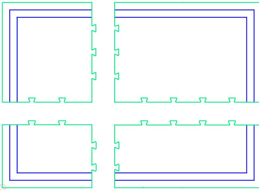
The generic DXF output in the ejection rubber menu now has a checkbox for arcs, so if a machine does not support arcs a straight line only version can be output.
